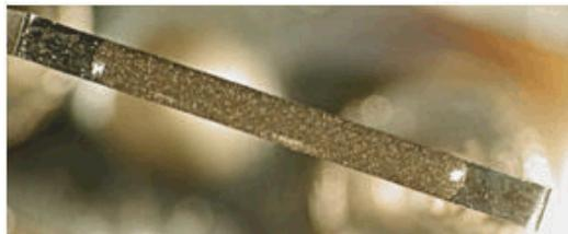
FIGURE 3.  $\text{LaB}_6$ /PIE mixture affixed to a filament.
