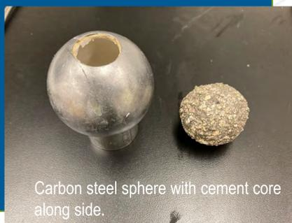
Carbon steel sphere with cement core along side.
