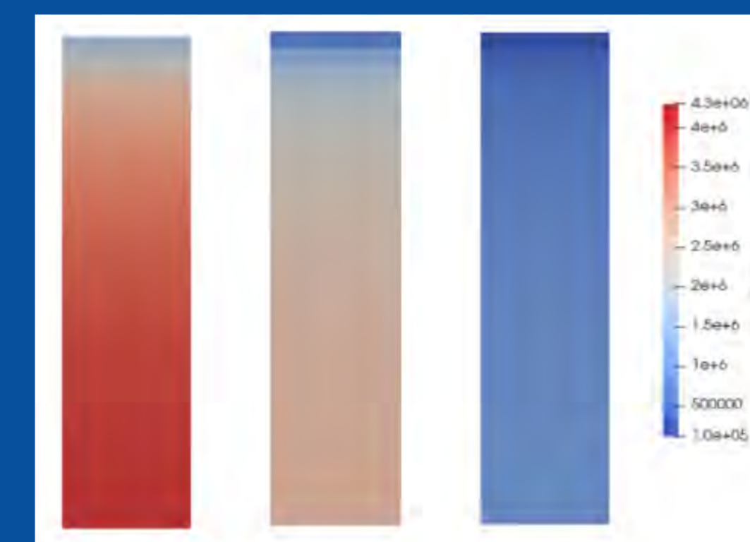
Figure 6: Snapshots of computational fluid dynamic simulation of CT4 with initial pressure of 4.3 MPa
