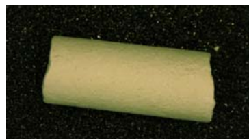
FIGURE 5. Portion of sintered \text{CeO}_2 rod originated from a Dry-Bag Isostatic Pressed, long “green” rod.
