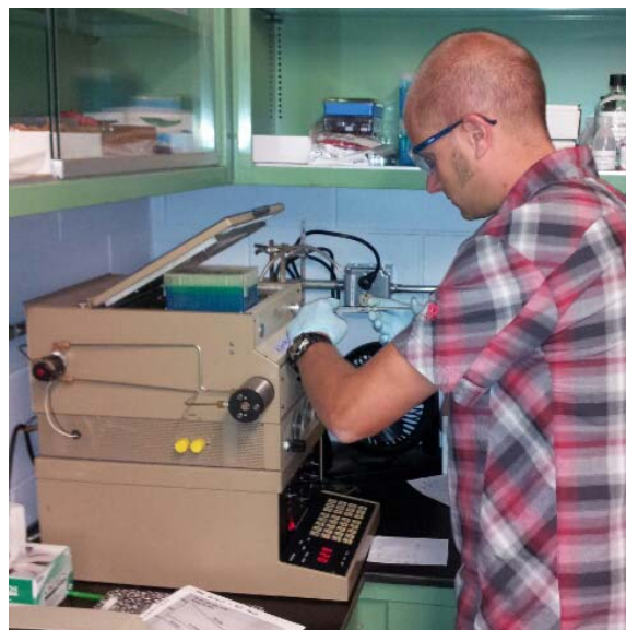
Figure 2. Ed Stowe, University of Idaho graduate student (a) analyzing biogas on gas chromatograph/thermal conductivity and (b) processing samples from a manure AD/fermenter system.
