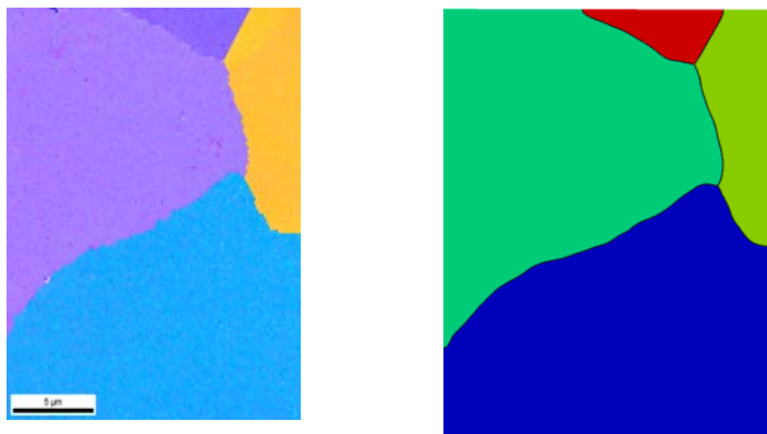
Figure 1. Microstructure reconstruction in MARMOT of a high burnup MOX fuel, where the EBSD scan is shown on the left and the reconstruction is shown on the right.
