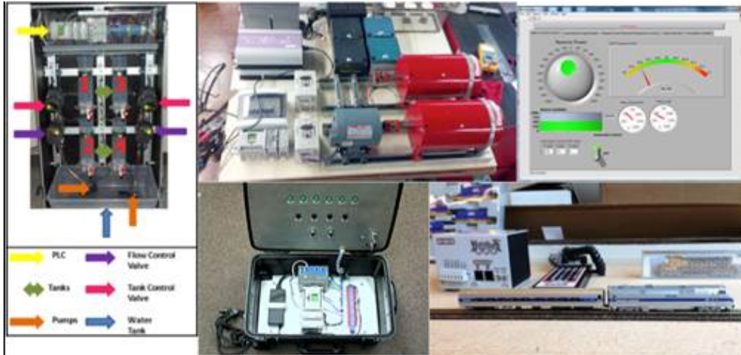
Figure 1. A collage of the enhancements to the testbed for machine learning security experiments include: (clockwise from top left) four tank control, Grid in a Box prototype, control screen for Grid in a Box, the scale model layout of train, and the environmental control system.
