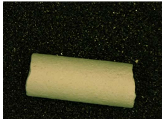
Figure 6. Right: Portion of sintered CeO 2 rod originated from a dry bag isostatic-pressed, long “green” rod.
