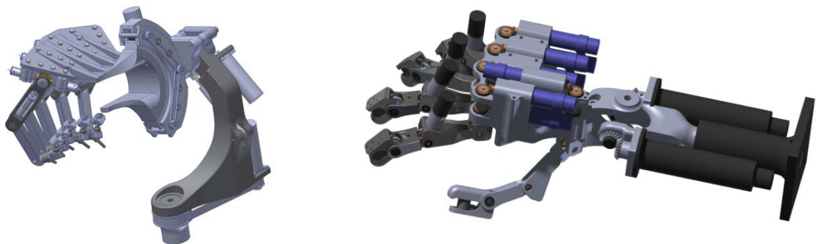
Figure 1. Image of haptic user interface and corresponding robotic hand.
