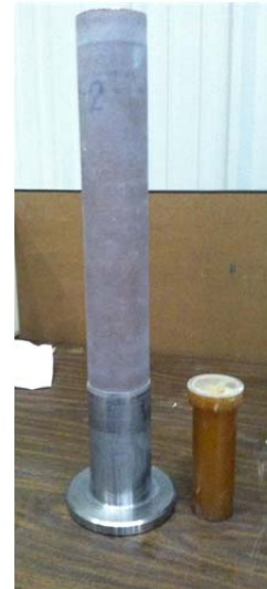
Figure 3. Larger bag tool assembly with smaller, inner parts bag. (The powder is poured into this bag which is then inserted into the assembly prior to isostatically pressing the rod.)
