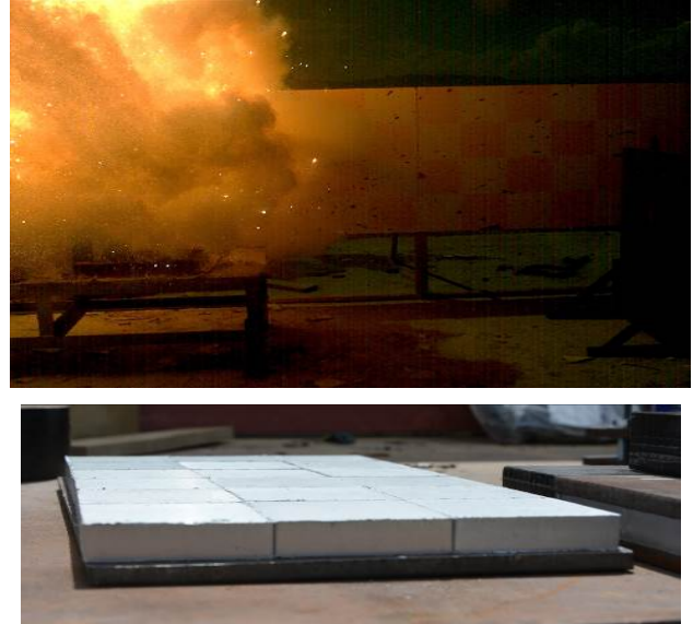
Figure 2. Semi-energetic targets were ignited by the impact of an incoming projectile.
