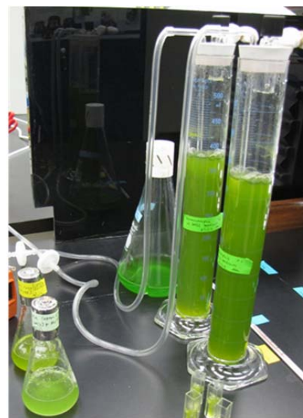
Figure 1. Photobioreactors and shake flasks used for single and mixed culture studies.
