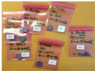
CeO 2 pellets produced using SPS
