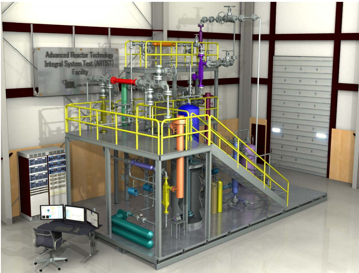
Figure 1. Rendering of a computer-aided design model showing the ARTIST capability in the INL Energy Systems Laboratory (ESL).
