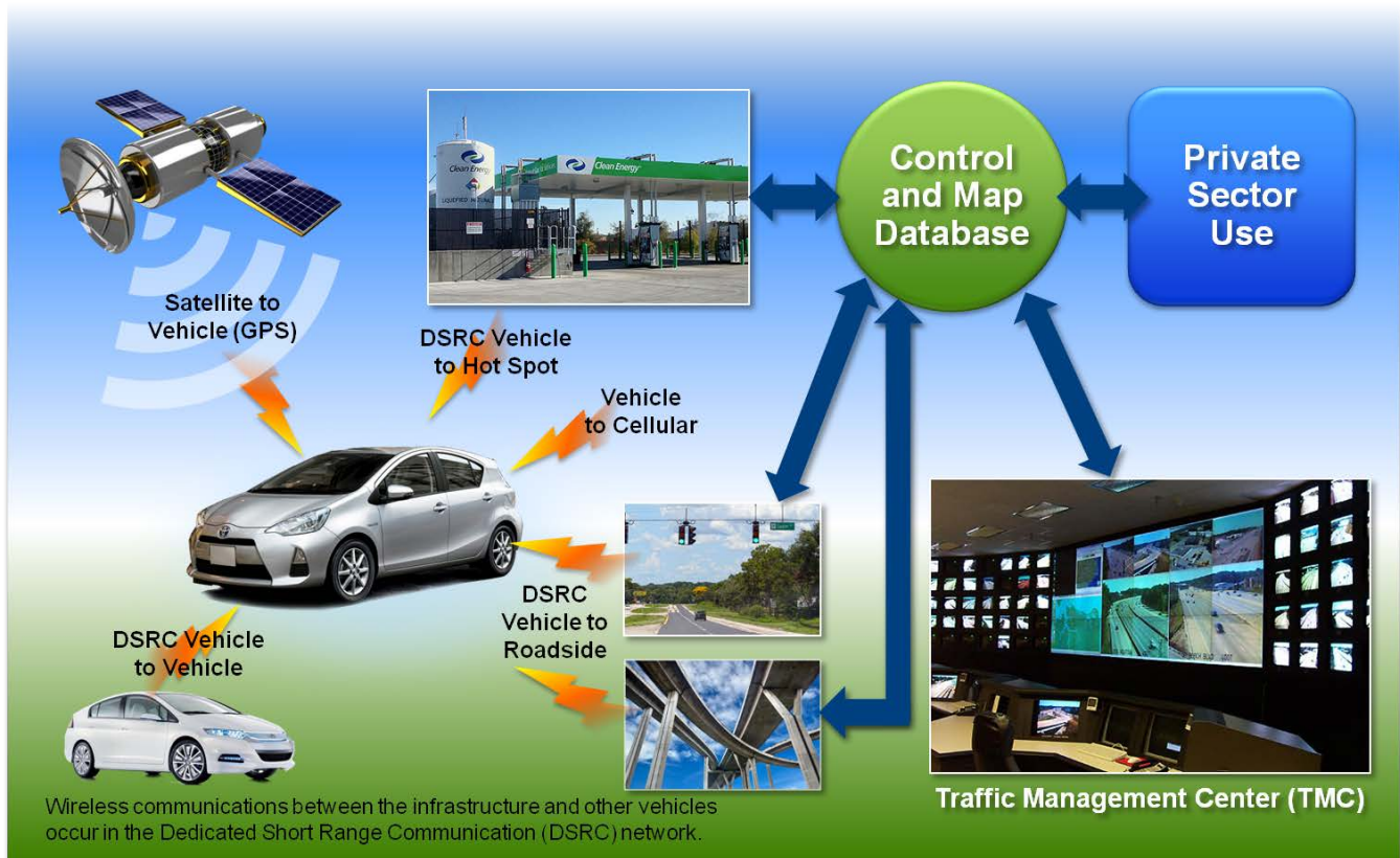
Figure 1. Overview of vehicle-to-vehicle and vehicle-to-infrastructure interconnects.
