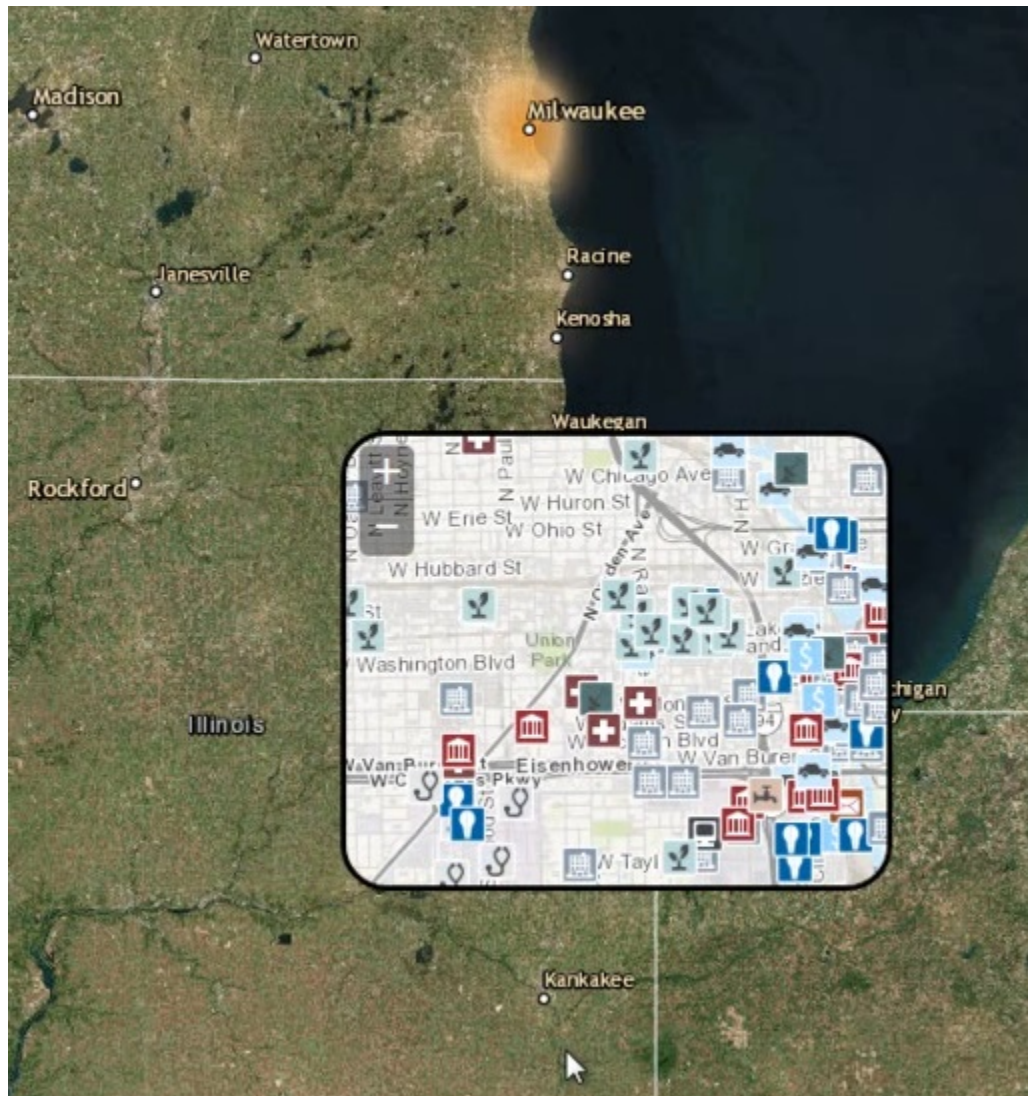
Figure 2. Spyglass tool for examining local detail over a regional overview map. Individual CI assets near downtown Chicago are visible in the spyglass, which has been zoomed to a large relative scale and centered on the regional map over Chicago.
