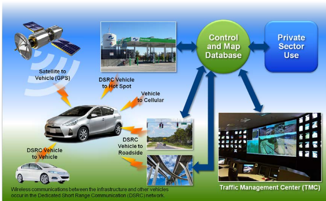
Figure 1. Overview of vehicle-to-vehicle and vehicle-to-infrastructure.
