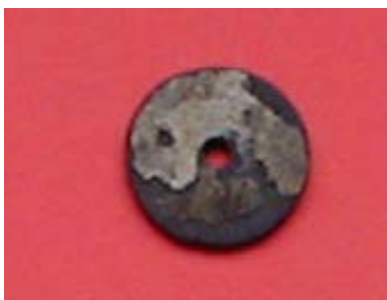
Figure 5. State of the reduced pellet, partial silvery white color on the surface of the reduced pellet was solidified calcium chloride (electrolysis temperature = 900^{\circ}\text{C} , electrolysis duration = 31 hours).
