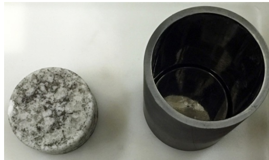
Figure 2. FLiNaK ingot and glassy carbon crucible.
