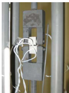
Figure 3. The experimental setup for delayed hydride cracking experiments. The furnace enclosing the sample and grip attachments is not shown in this figure.
