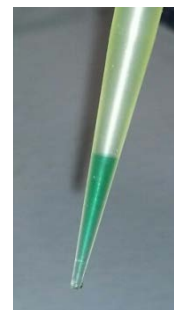
Figure 1. UO_2 dissolved in EMImFHF.
