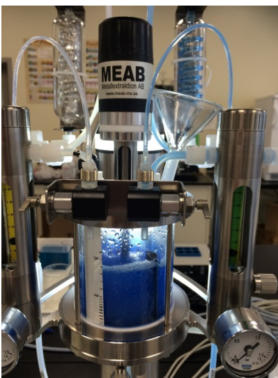
Figure 1. Lamp oil/acidic water experiment in AKUFVE.
