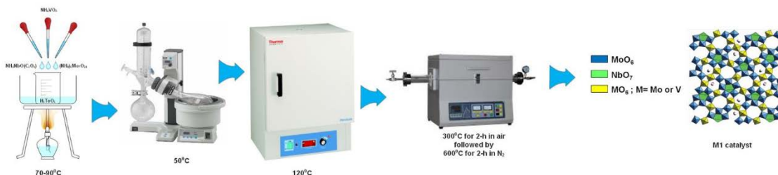
Figure 1. M1 catalyst synthesis by dry-up method.
