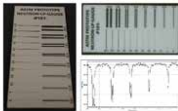
A picture of the prototype gauge (left), a neutron radiograph of the gauge (top right) and an example line profile (bottom right) showing the contrast between lines from a series line pairs.
