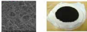
Figure 5. SEM image (left) and general image of PDMS/CNT membrane (right).
