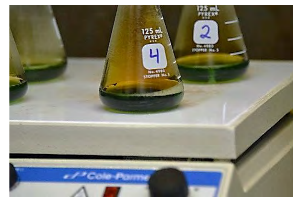
Traditional hot plate dissolution in the ARL
