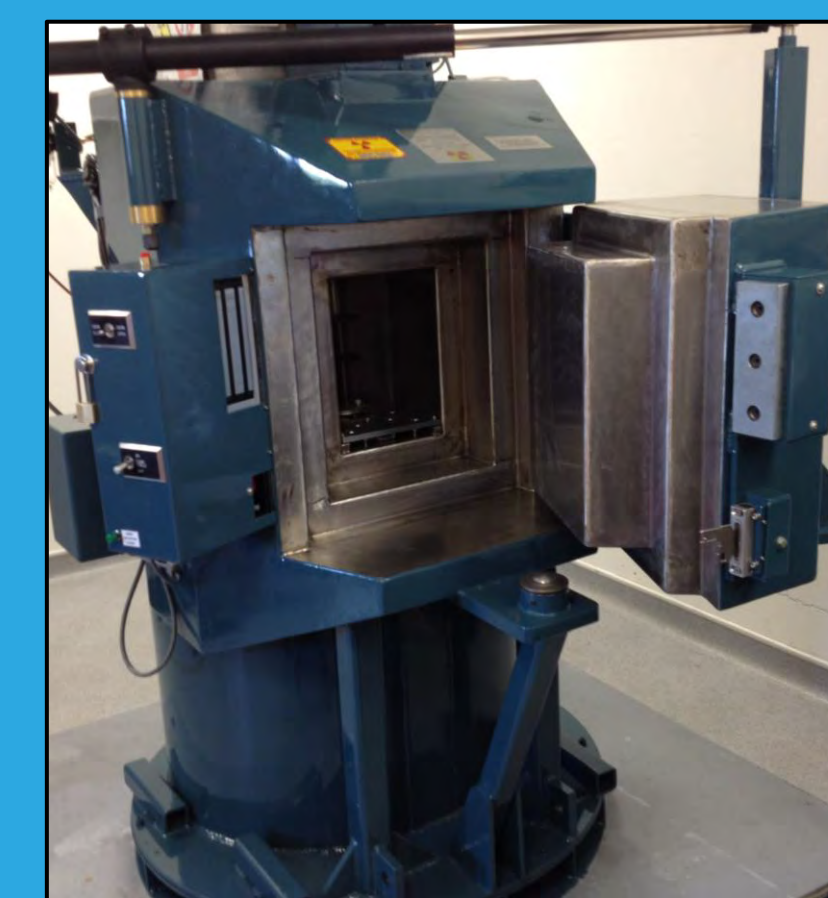
Foss Therapy Services Model 812 Cobalt-60 Gamma Irradiator
